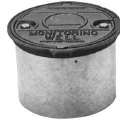
Covers and rings may be ordered painted white with a black triangle. Manholes with heavy duty skirts, welded skirts, as well as the fully cast 519 series manholes shown below are also available. All Morrison manholes have been independently tested to meet AASHTO standard for "H-20" truck loadings, ASTM A48, and section 206-3 of the American Public Works Association. Each manhole is individually boxed.
