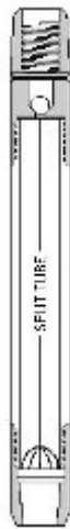
Standard Split Barrel Sampler Assembly Head (Top), Split Barrel (Center) & Shoe with Trap (Bottom)
